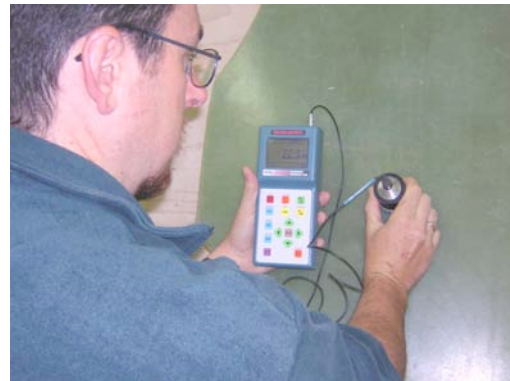
Fig 9: Ultrasonic Testing of FRP
