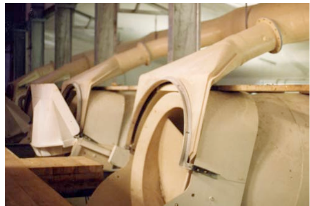
Fibreglass lip extraction hoods on pelt and hide processors.
