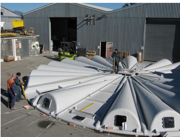
Segmented fibreglass covers are trial assembled at ARMATEC factory before despatch. This ensures dimensions are correct, and minimises installation time and difficulties at site.
